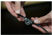
22. Turn barrel adjuster 1-2 full turns counter-clockwise (outward) to remove all slack from inner cable
