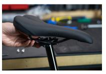
5. Reach in from the front or rear with your index finger to support one of the barrel nuts and insert one of the clamp bolts up from the bottom and thread a few turns into the nut
