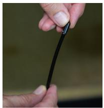
14. Insert inner cable through cable barrel and begin inserting cable through outer housing from seat tube end until there are just a few inches/cm protruding from the outer housing
