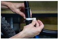
4. Remove dropper post from frame, measure and record distance from mark on lower tube to end of actuator cable receptacle
