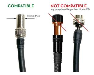
**Note:** Connecting the pump will reduce the pressure by 30-50 PSI as the air volume is very small. Example: if you connect the pump and the gauge reads 200 PSI, your post was at 230-250 PSI before you connected the pump. Always re-inflate to the correct pressure before removing the pump. Removing the pump will not reduce the pressure inside the post.
