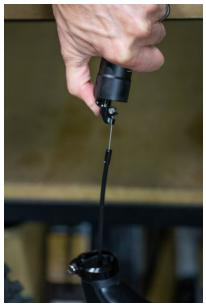
17. Push dropper post downward until end cap on outer housing is fully engaged with socket on post actuator
