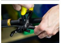
11. Cut the outer housing at the mark
