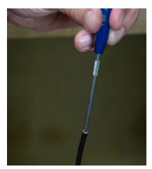
13. Install supplied end caps (ferrules) on each end of the outer housing
