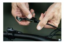
23. Insert dropper post into frame up to height marked in step 3 while pulling on outer cable housing as needed to move it smoothly through the frame
