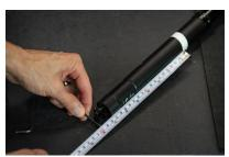
5. Insert outer cable housing through frame until it is flush with the top of the seat collar
