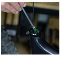
16. Insert barrel into actuator arm of dropper post – this requires partially actuating the arm
