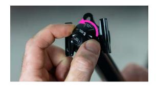
3. Use hollow XZN16 socket (available from Wolf Tooth) to remove lockring. Hold lower cradle with parallel-jaw pliers wrench such as Knipex 86 03 250 (ideal), adjustable wrench, or 27mm open-end wrench.
