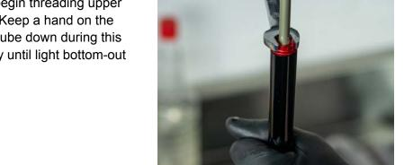
43. Remove cartridge from vise soft-jaws. Holding lower cap with pliers-wrench, lightly tighten the upper cylinder cap using 13mm open-end wrench. Upper cap does not require much torque, only contact plus 1/8 turn.
