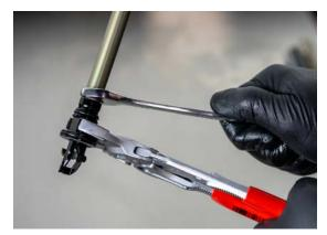
20. Remove valve body assembly from lower cap by gently gripping with pliers wrench and pulling upwards.
