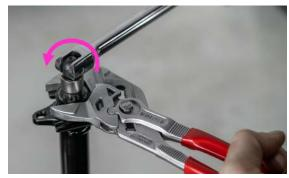
4. Pull up firmly to remove lower cradle from stanchion. If the low cradle sticks to the stanchion, tap upward with plastic faced hammer.
