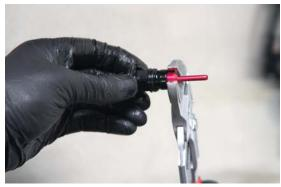
21. Gently insert 2.5mm ball-end hex key through top of needle to extract poppet valve from valve body.
