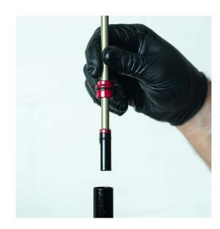
17. Remove cartridge from vise and pour fluid contents from cylinder and reservoir into a graduated cylinder. In droppers bought before Jan of 2023 the fluid should be clear with a yellow tint and purchased after the fluid will have a blue tint. Fluid should be free of suspended solids. Discolored or contaminated fluid should be discarded into a waste oil container.
