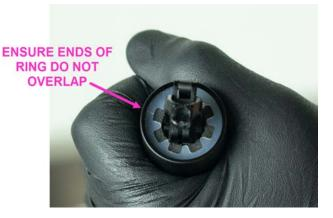
23. Use internal snap ring pliers to install snap ring. Ensure that snap ring is fully seated into its gland (will typically have an audible snap sound when it fully seats and should rotate easily when pulled by one of the "ears").
