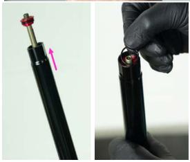
28. Apply a small amount of grease to inside of lower cradle, and install onto top of stanchion in orientation shown. Note the orientation relative to the laser markings on the lower tube - the RIGHT pivot block on the lower cradle assembly is marked with an R, while the laser marked graphics on the housing are on the backside of the post.
