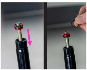
6. Use 7mm open-end wrench to hold piston rod. Remove rod-end cap using 13mm cone wrench.
