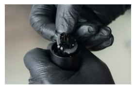
48. Install plastic filter retaining ring. Use a pick to push the retaining ring into position, ensuring that the split ends do not overlap (overlap will prevent installation of snap ring).
