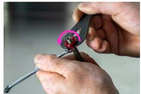
7. Use internal snap-ring pliers to remove snap-ring from bottom of post.
