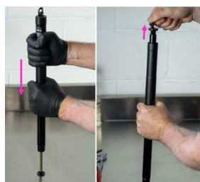
10. Slide stanchion out of bottom of lower tube. Be careful not to lose the brass anti-rotational pins as they are removed with the stanchion.
