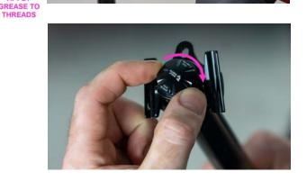
31. Reinstall saddle, upper cradle, spherical bolts and threaded barrels, and return saddle to original position. Torque bolts to 6 Nm.
