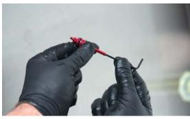
22. Remove and replace the two o-rings on the poppet valve (1.5 X 2.0, 1.5 X 2.5).
