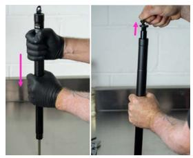
10. Connect shock pump to Schrader valve at top of cartridge piston rod. With cartridge held vertically (Schrader valve at highest point), use bleed valve on shock pump to slowly release pressure from cartridge reservoir.
