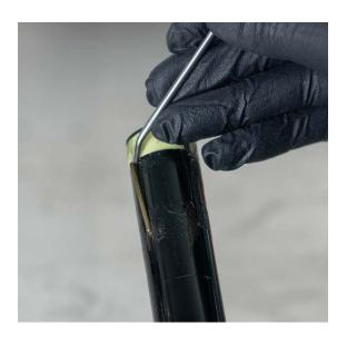
12. Remove wiper seal. Clean and inspect for any damage to seal lip. Replace wiper seal if any damage is found. Replacement of wiper seal is recommended every 100 hours or as needed
