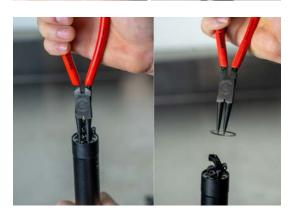
8. Use a pick to unseat and remove plastic air filter retainer ring.
