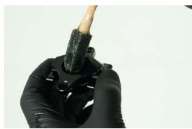
29. Apply small amount of grease to threads of lockring and install to secure lower cradle in place. Hold lower cradle using parallel-jaw pliers wrench, and use hollow XZN16 socket and 3/8"-drive torque wrench to torque lockring to 35 Nm (26 lb-ft).
