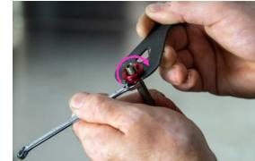
27. Extend stanchion until rod end-cap is seated into position. Place the 1.5x16.5mm o-ring onto the top of the rod end-cap.
