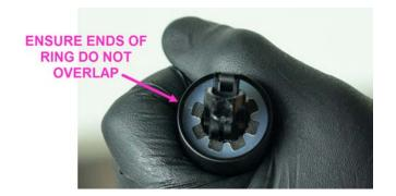
49. Use internal snap ring pliers to install snap ring. Ensure that snap ring is fully seated into its gland (will typically have an audible snap sound when it fully seats).
