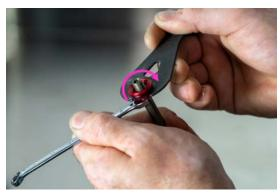
51. Extend stanchion until rod end-cap is seated into position. Place a new 1.5x16.5mm o-ring onto the top of the rod end-cap, seating o-ring fully into position.
