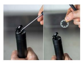
Reinstall air cap on end of piston rod. Push end of piston rod against workbench firmly to unseat the cartridge. Remove the air cap and slide the cartridge out of the housing.
