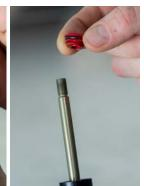
7. Use internal snap-ring pliers to remove snap-ring from bottom of post.
