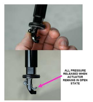
13. Begin unthreading upper cylinder cap. Hold cartridge by flats on lower cylinder cap using Knipex pliers wrench or 15mm open-end wrench. Use 13mm open-end wrench on upper cylinder cap to break cap loose, but do not yet fully remove.
