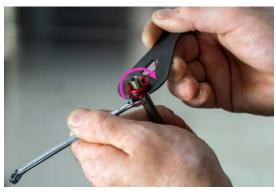
25. Extend stanchion until rod end-cap is seated into position. Place the 1.5x16.5mm o-ring onto the top of the rod end-cap. Inspect o-ring for damage and replace if necessary.
