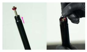
26. Apply a small amount of grease to inside of lower cradle, and install onto top of stanchion in orientation shown. Note the orientation relative to the laser markings on the lower tube - the RIGHT pivot block on the lower cradle assembly is marked with an R, while the laser marked graphics on the housing are on the backside of the post.
