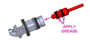
36. Place cylinder over valve body and thread into lower cap. Only one end of cylinder has wrench flats - this end should be threaded into lower cap.
