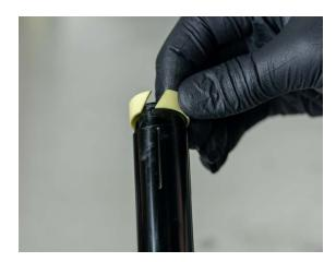
15. Install wiper seal into top of lower tube. Apply a light coat of grease to inside of wiper seal. We recommend a new wiper seal every year or 100 hours of use.
