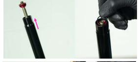
52. Apply a small amount of grease to inside of lower cradle, and install onto top of stanchion in orientation shown. Note the orientation relative to the laser markings on the lower tube - the RIGHT pivot block on the lower cradle assembly is marked with an R, while the laser marked graphics on the housing are on the backside of the post.
