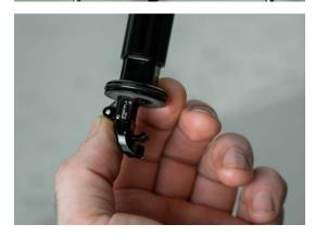
12. **IMPORTANT** - Verify that no remaining pressure is contained in the cartridge - actuator valve will remain in open state when all pressure has been released.
