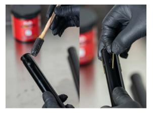
19. Install split bushing onto bottom of stanchion.
