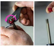
7. Use internal snap-ring pliers to remove snap-ring from bottom of post.
