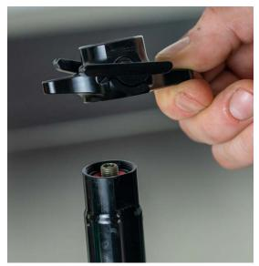
Slide stanchion down to expose piston rod end cap.
