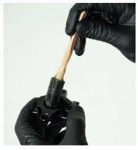
27. Apply small amount of grease to threads of lockring and install to secure lower cradle in place. Hold lower cradle using parallel-jaw pliers wrench, and use hollow XZN16 socket and 3/8"-drive torque wrench to torque lockring to 35 Nm (26 lb-ft).
