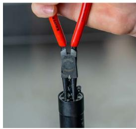
26. Install piston rod end-cap onto end of piston rod in orientation shown. Hold piston rod with 7mm open-end wrench, lightly torque end-cap using 13mm cone wrench.
