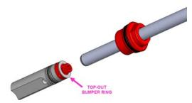
33. Use 1.95mm gauge pin or 1.5mm hex key to hold piston coupler. Using a 7mm open-end wrench or a crow's foot attachment on a torque wrench to torque piston rod to 2.0 Nm.
