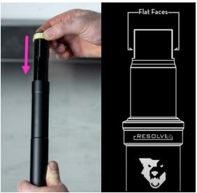
21. Install cartridge into housing assembly. Push firmly on end of actuator until cartridge is full seated (audible thud upon engagement).
