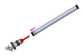
37. Hold lower cap using pliers wrench or 15mm open-end wrench. Using 14mm open-end wrench to tighten cylinder onto lower cap. Torque to 7.0 Nm.
