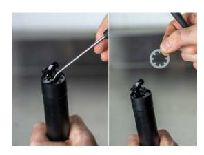
Reinstall air cap on end of piston rod. Push end of piston rod against workbench firmly to unseat the cartridge. Remove the air cap and slide the cartridge out of the housing.
