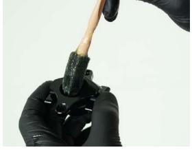
53. Apply small amount of grease to threads of lockring and install to secure lower cradle in place. Hold lower cradle using parallel-jaw pliers wrench, and use hollow XZN16 socket and 3/8"-drive torque wrench to torque lockring to 35 Nm.
