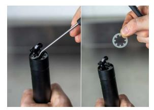
Reinstall air cap on end of piston rod. Push end of piston rod against workbench firmly to unseat the cartridge. Remove the air cap and slide the cartridge out of the housing.
