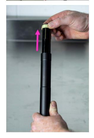
11. Remove brass pins from stanchion. Wipe clean and set aside. If replacing pins are needed - take note of diameter of each pin. Replacement pins are available in 4 diameters, ranging from 1.96mm to 2.02mm. Pin diameter may be determined by presence of cut rings on the side of the pin (see illustration).
