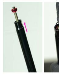
28. Apply a small amount of grease to inside of lower cradle, and install onto top of stanchion in orientation shown. Note the orientation relative to the laser markings on the lower tube - the RIGHT pivot block on the lower cradle assembly is marked with an R, while the laser marked graphics on the housing are on the backside of the post.
