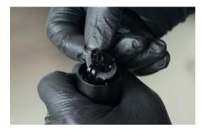
48. Install plastic filter retaining ring. Use a pick to push the retaining ring into position, ensuring that the split ends do not overlap (overlap will prevent installation of snap ring).
