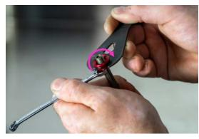
27. Extend stanchion until rod end-cap is seated into position. Place the 1.5x16.5mm o-ring onto the top of the rod end-cap.
