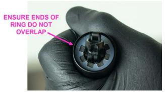
25. Use internal snap ring pliers to install snap ring. Ensure that snap ring is fully seated into its gland (will typically have an audible snap sound when it fully seats and should rotate easily when pulled by one of its "ears").
