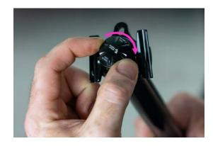
30. Reconnect cable from dropper lever, and reinstall post into frame.
