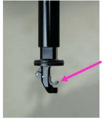
ALL PRESSURE RELEASED WHEN ACTUATOR REMAINS IN OPEN STATE
