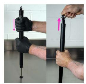
10. Connect shock pump to Schrader valve at top of cartridge piston rod. With cartridge held vertically (Schrader valve at highest point), use bleed valve on shock pump to slowly release pressure from cartridge reservoir.
