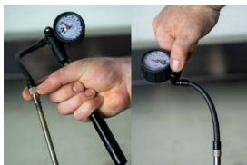
11. Manually open the actuator valve at the bottom of the cartridge to release any remaining pressure contained in the cartridge cylinder into the reservoir. Release this pressure from the reservoir with the shock pump bleeder valve.
