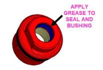
31. Slide cylinder cap assembly back onto non-threaded end of piston rod.
