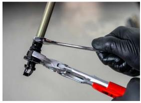
20. Remove valve body assembly from lower cap by gently gripping with pliers wrench and pulling upwards.
