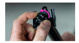
Use hollow XZN16 socket (included in dropper post packaging) to remove lockring. Hold lower cradle with parallel-jaw pliers wrench such as Knipex 86 03 250 (ideal), adjustable wrench, or 27mm open-end wrench.
