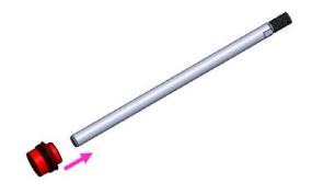
32. Place a new top-out bumper ring over threaded boss of piston coupler, and thread piston rod onto coupler. Ensure that top-out bumper is not pinched between piston rod and coupler. Top-out ring should turn freely after piston rod and coupler are attached.
