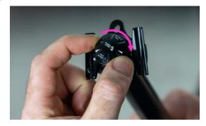
31. Reinstall saddle, upper cradle, spherical bolts and threaded barrels, and return saddle to original position. Torque bolts to 6 Nm.
