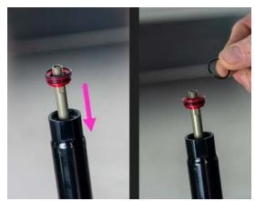
6. Use 7mm open-end wrench to hold piston rod. Remove rod-end cap using 13mm cone wrench.
