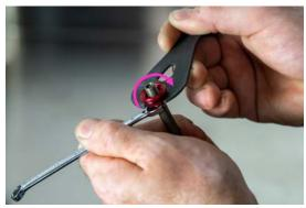
25. Extend stanchion until rod end-cap is seated into position. Place the 1.5x16.5mm o-ring onto the top of the rod end-cap. Inspect o-ring for damage and replace if necessary.
