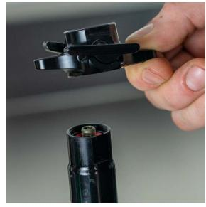
5. Slide stanchion down to expose piston rod end cap. Remove upper o-ring and set aside.
