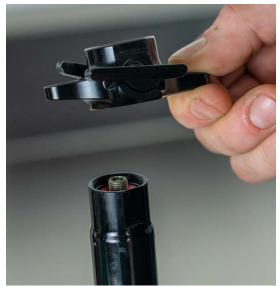
Slide stanchion down to expose piston rod end cap.
