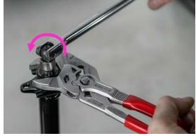
4. Pull firmly upward to remove lower cradle from stanchion.
