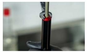
20. Tighten cylinder cap using 13mm open-end wrench. This step should be performed with cartridge removed from vise. Hold lower cap wrench flats during tightening with Knipex pliers wrench or 15mm open-end wrench. Tighten ⅓ turn past contact.
