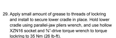
\*\*\* always use a torque wrench for lock ring installation. Under or over torquing this part is a potential safety issue \*\*\*
