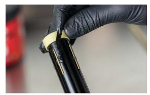
20. Slide stanchion with bushing and pins into lower tube. Pay attention to orientation of stanchion relative to lower tube - the flats on the top of the stanchion are the left and right sides, while the lower tube laser markings are located on the backside. Ensure that pins engage into the lower tube channels without binding. Slide stanchion to full extension, check for any binding or excess lash.
