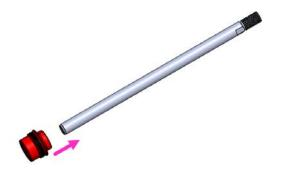
32. Place a new top-out bumper ring over threaded boss of piston coupler, and thread piston rod onto coupler. Ensure that top-out bumper is not pinched between piston rod and coupler. Top-out ring should turn freely after piston rod and coupler are attached.
