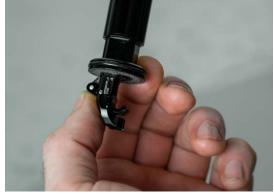
12. **IMPORTANT** - Verify that no remaining pressure is contained in the cartridge - actuator valve will remain in open state when all pressure has been released.
