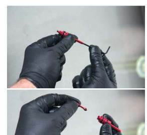
22. Remove and replace the two o-rings on the poppet valve (1.5 X 2.0, 1.5 X 2.5).
