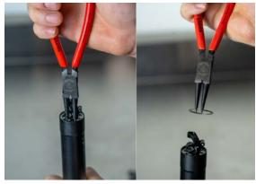
8. Use a pick to unseat and remove plastic air filter retainer ring.
