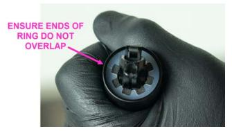
25. Use internal snap ring pliers to install snap ring. Ensure that snap ring is fully seated into its gland (will typically have an audible snap sound when it fully seats and should rotate easily when pulled by one of its "ears").
