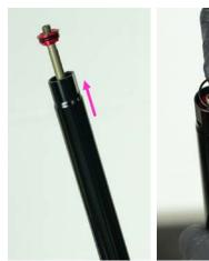
28. Apply a small amount of grease to inside of lower cradle, and install onto top of stanchion in orientation shown. Note the orientation relative to the laser markings on the lower tube - the RIGHT pivot block on the lower cradle assembly is marked with an R, while the laser marked graphics on the housing are on the backside of the post.
