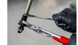
20. Remove valve body assembly from lower cap by gently gripping with pliers wrench and pulling upwards.
