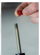
7. Use internal snap-ring pliers to remove snap-ring from bottom of post.
