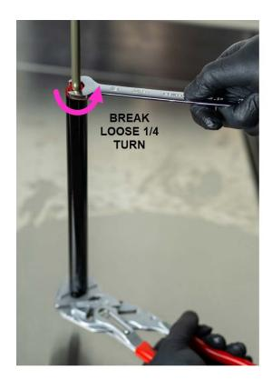
14. With plastic soft jaws in place, clamp actuator at bottom of cartridge in vise, holding the cartridge in an upright state. Be careful not to over-clamp.
