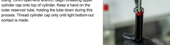
43. Remove cartridge from vise soft-jaws. Holding lower cap with pliers-wrench, lightly tighten the upper cylinder cap using 13mm open-end wrench. Upper cap does not require much torque, only contact plus 1/8 turn.
