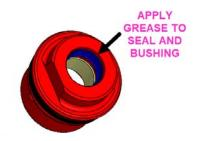
31. Slide cylinder cap assembly back onto non-threaded end of piston rod.
