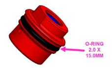
30. Apply suspension grease to inside of u-cup (blue seal) and bushing.
