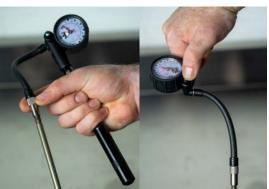
pressure from the reservoir with the shock pump bleeder valve.
