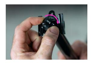
30. Reconnect cable from dropper lever, and reinstall post into frame.
