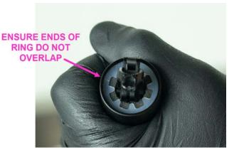
23. Use internal snap ring pliers to install snap ring. Ensure that snap ring is fully seated into its gland (will typically have an audible snap sound when it fully seats and should rotate easily when pulled by one of the "ears").
