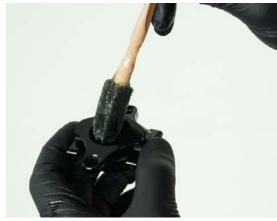
53. Apply small amount of grease to threads of lockring and install to secure lower cradle in place. Hold lower cradle using parallel-jaw pliers wrench, and use hollow XZN16 socket and %"-drive torque wrench to torque lockring to 35 Nm.
