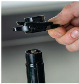
5. Slide stanchion down to expose piston rod end cap. Remove upper o-ring and set aside.
