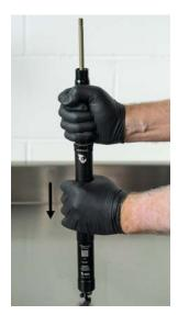
22. Check that foam air filter is seated in place, and install plastic filter retaining ring. Use a pick to push the retaining ring into position, ensuring that the split ends do not overlap (overlap will prevent installation of snap ring). NOTE: filter should be replaced every year or 100 hours of use.
