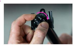
31. Reinstall saddle, upper cradle, spherical bolts and threaded barrels, and return saddle to original position. Torque bolts to 6 Nm.
