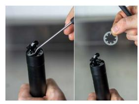
9. Reinstall air cap on end of piston rod. Push end of piston rod against workbench firmly to unseat the cartridge. Remove the air cap and slide the cartridge out of the housing.
