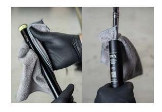
14. Remove split bushing from bottom of stanchion. Wipe bushing clean.
