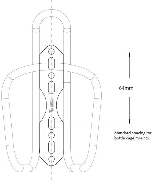
Print and fold on dotted line. Line up dash & dot holes to frame mounts.
