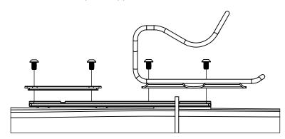
**STEP 4.** Tighten frame screws to manufacturers recommended torque (See notes). Check clearances with bottle case and accessories installed before riding
