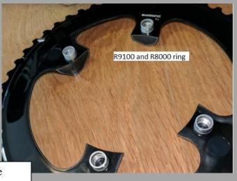
Lay the ring on to the Wolf Tooth Shimano Asymmetric 110 \* Be sure to align the clocking tab with the anti-chain jam peg
