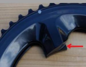
Scribe a line into the Wolf Tooth ring using the Original ring as a guide. With a little filing you should end up with a good looking fit.
