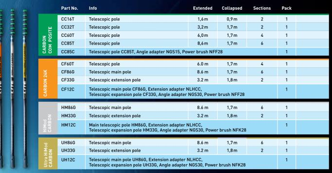
All telescopic poles (excl. extension poles) are delivered with an internal hose (pole length + approx. 30 cm)
