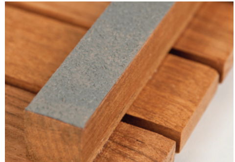
rubberized strips on the footing
