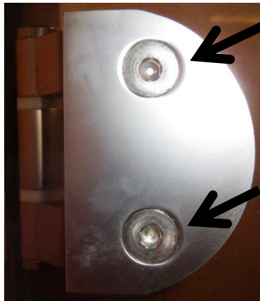
Loosen the screws slightly
