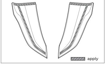
A-3. Fold a small tail of the red backing material from the [ $3M^{TM}$  Double-Sided Tape] and secure it with masking tape so that the backing material is accessible.
