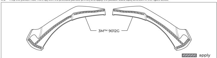
Fold a small tail of the red backing material from the [ $3M^{\text{IM}}$  Double-Sided Tape] and secure it with masking tape so that the backing material is accessible.
