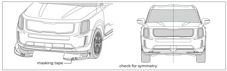
B-2. Once it is properly aligned, pull the tails on the double-sided tape and firmly press along the taped areas to ensure proper adhesion.
