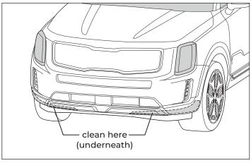
Prep the [carbon fiber front lip] with the provided [surface primer] and apply the [double-sided tape] as shown in the figure below.
