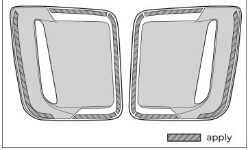
A-4. Ensure that your Telluride's front bumper has been thoroughly cleaned and prep it with the provided [surface primer]. \*Be careful not to overuse the primer as it may damage the paint job.
