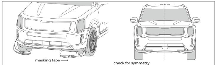
B-2. Once it is properly aligned, pull the tails on the double-sided tape and firmly press along the taped areas to ensure proper adhesion.
