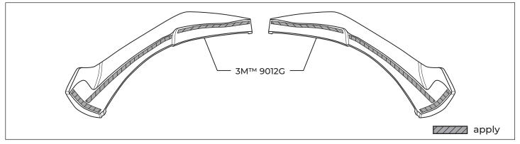
A-3. Fold a small tail of the red backing material from the [3M<sup>TM</sup> Double-Sided Tape] and secure it with masking tape so that the backing material is accessible.
