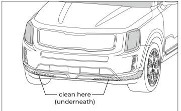
A-2. Prep the [carbon fiber front lip] with the provided [surface primer] and apply the [double-sided tape] as shown in the figure below.
