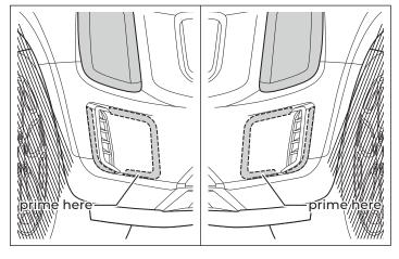
B-2. Once it is properly aligned, pull the tails on the double-sided tape and firmly press along the taped areas to ensure proper adhesion. (Done)
