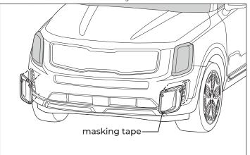
A-2. Prep the [carbon fiber front air ducts] with the provided [surface primer] and apply the [double-sided tape] shown in the figure below.
