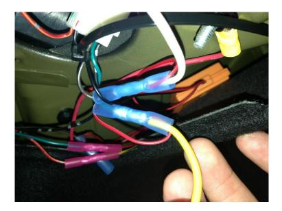
Route the Jumper wires up to the trunk lid. Look at the LEFT INNER trunk LED and locate to wires. 1 pink and 1 solid green. Cut both wires just like you did on the lower plug making sure to leave enough excess for easy crimping. Note my jumper wires were yellow and white, but in the picture below are black and red (exledusa pic) they are the same. Connect wires as follows:
