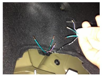
Now, I chose to use butt connectors for a clean, hassle free connection. You may solder, use crimps, etc.
