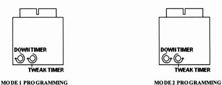
NOTE: If the module has already been powered up please unplug it, make the programming adjustments and wait at least 30 seconds before plugging the module back in.
