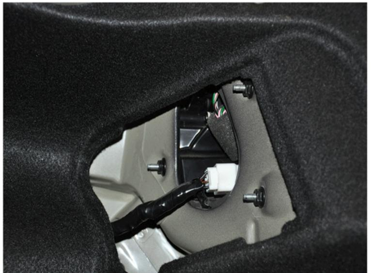
STEP 9: Remove (3) 10mm bolts holding in tail light
