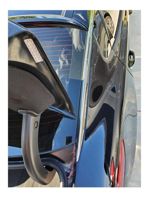
Now you have two options to route the wire inside the trunk, you could drill a hole through the body panel into the trunk and route the wire down in side the trunk. Hole could be just under the window where the wire comes out from under the window track. Or you can do what I did and route it along the body panel edge and use how glue gun
