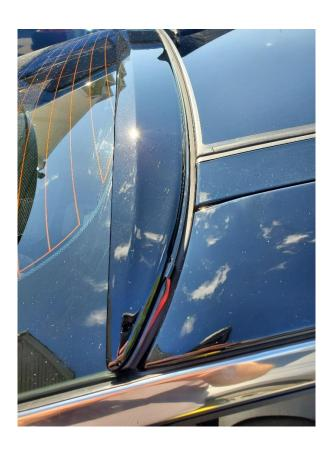
Once you have the wire routed over to the side window, you have to carefully push it under the window track going done the side of the car. It goes in easily in some areas, and some areas are a little harder. Keep working it until it is fully under the window track down the entire side.
