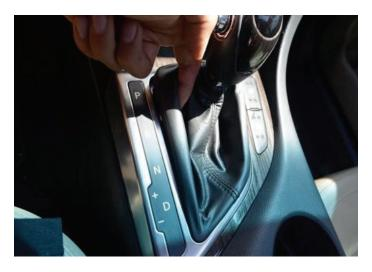
5. To remove the shifter knob, grab shifter knob, pull up and "wiggle" knob to release.
