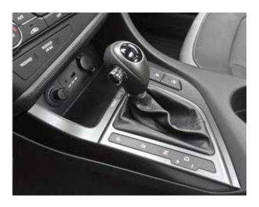
3. Start by removing the leather trim around shifter. Pull up with your fingers on the trim around the other edge of the leather.
