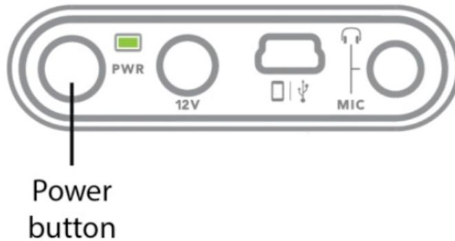
If the PWR LED doesn't glow green when powered on, connect your instrument to a power source using the included 12V power supply.
