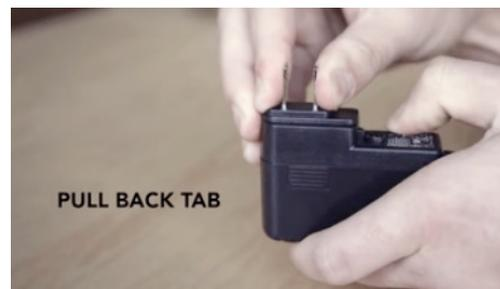
When assembled correctly, the prongs will sit flat with the body of the charger.
