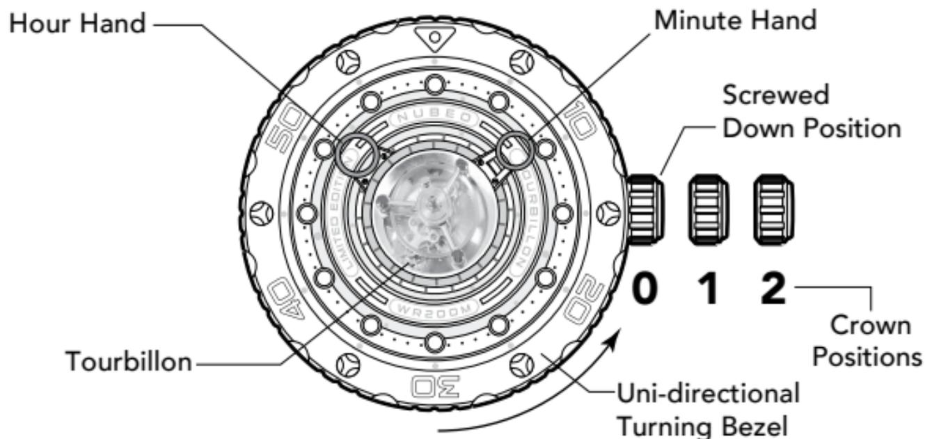
As your watch has a screw down crown feature, release the watch from the screw-down position before setting.
