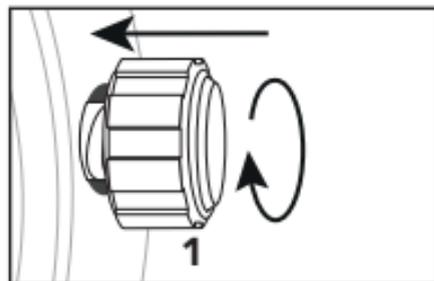
**TO SCREW:** Push the crown all the way in (towards the watch) then begin to turn clockwise until it is securely screwed down.
