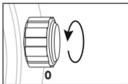
**TO UNSCREW:** Turn the crown anti-clockwise until it turns freely without tension. Gently pull the crown out to the other desired positions for watch setting (see specific operating instructions on the following pages).
