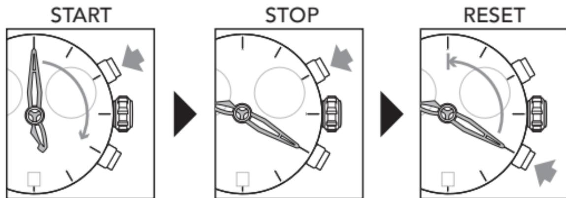
After 2 hours of continuous running, the chrono stops and resets automatically to save the battery.
