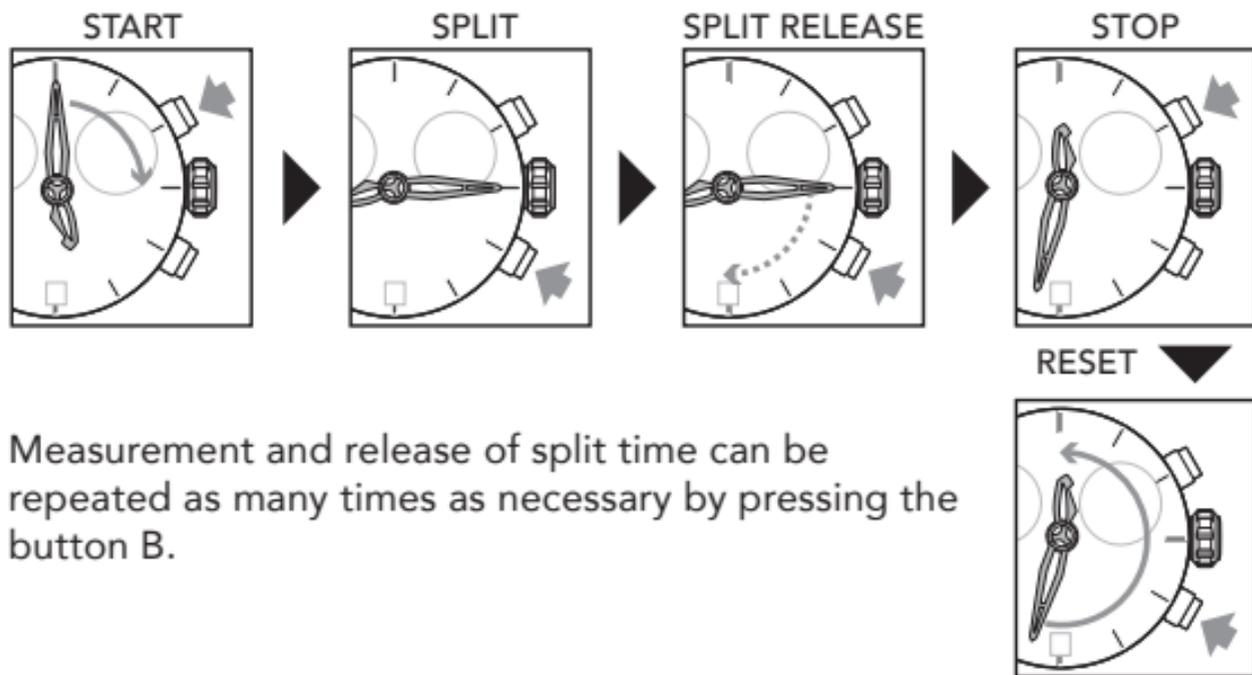
Measurement and release of split time can be repeated as many times as necessary by pressing the button B.
