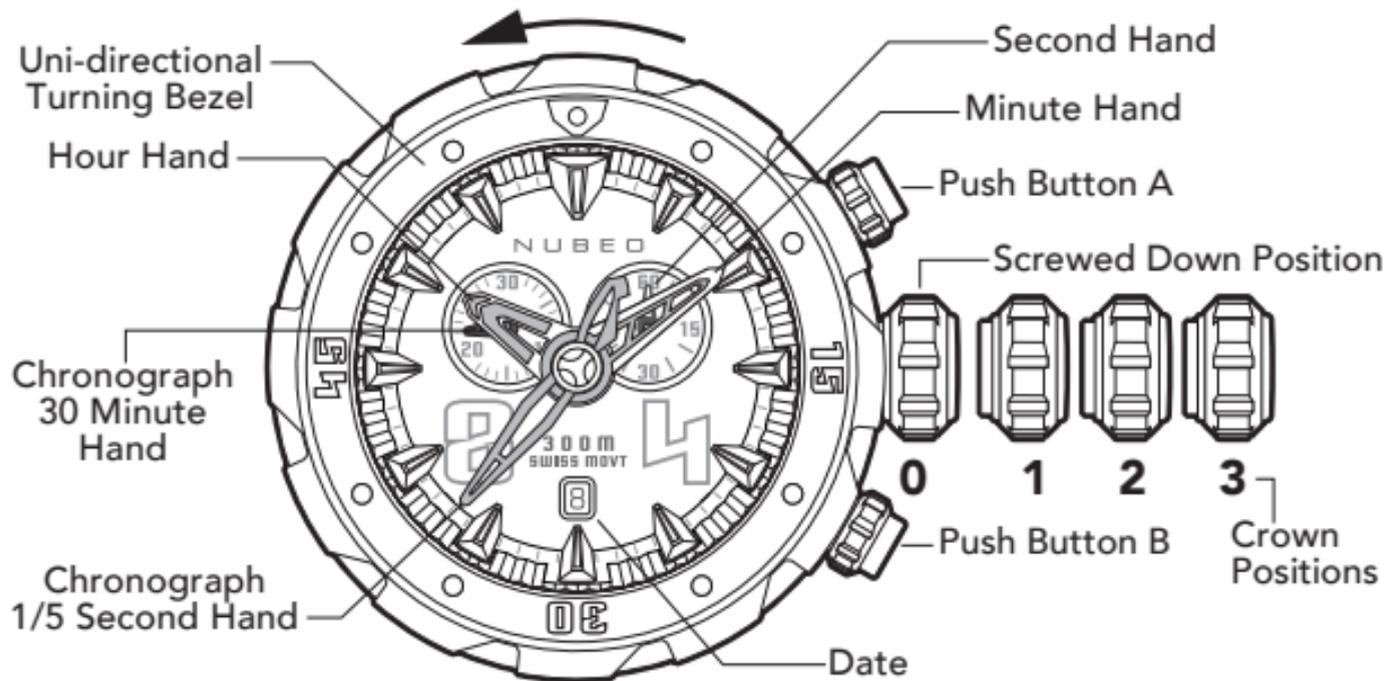
As your watch has a screw down crown feature, release the watch from the screw-down position before setting.
