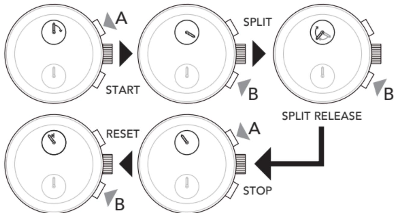
\* Measurement and release of the split time can be repeated as many times as necessary by pressing button B.
