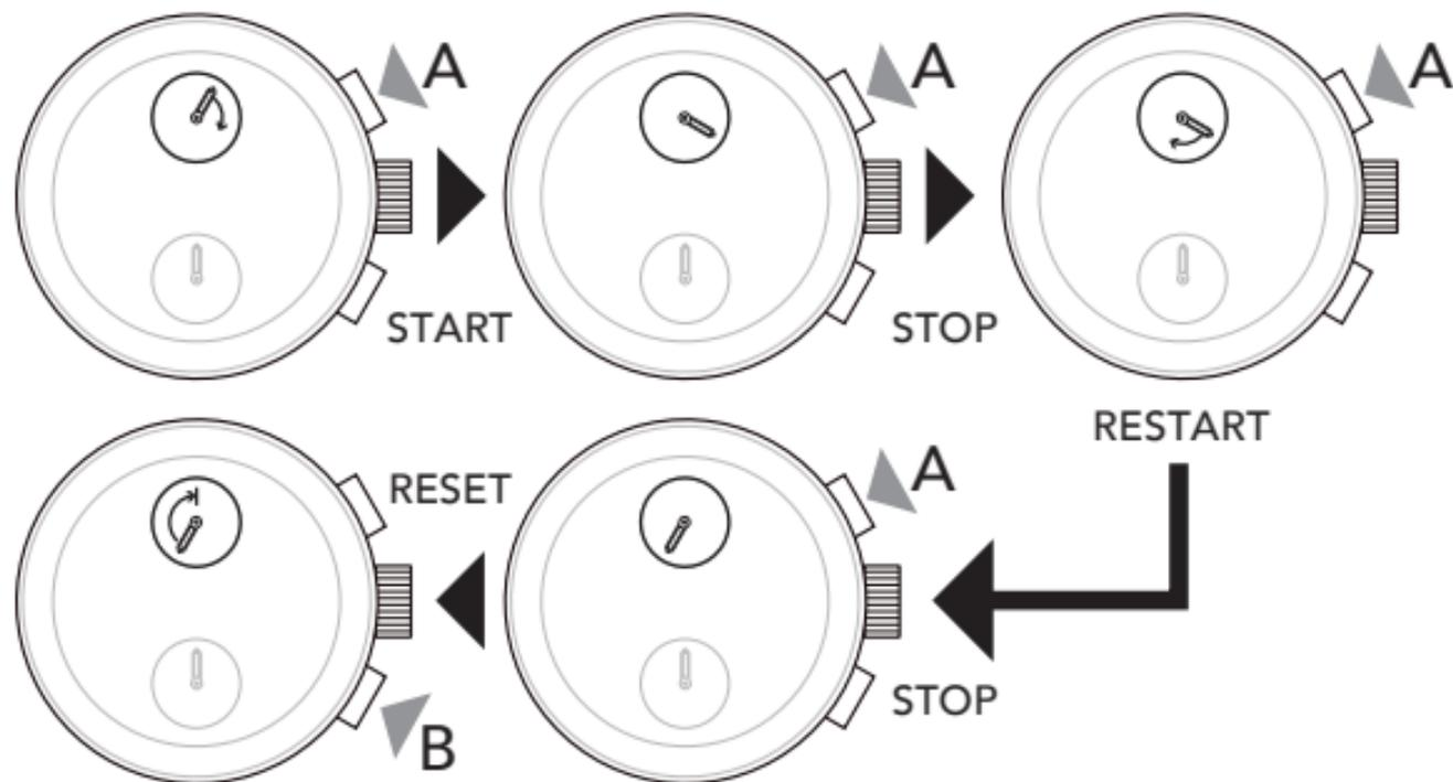
Restart and stop of the stopwatch can be repeated by pressing the button A.
