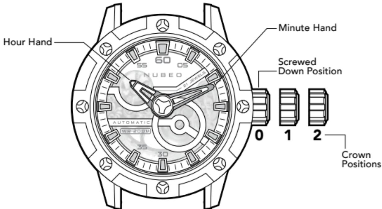
As your watch has a screw down crown feature, release the watch from the screw-down position before setting.
