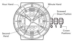
As your watch has a screw down crown feature, release the watch from the screw-down position before setting.
