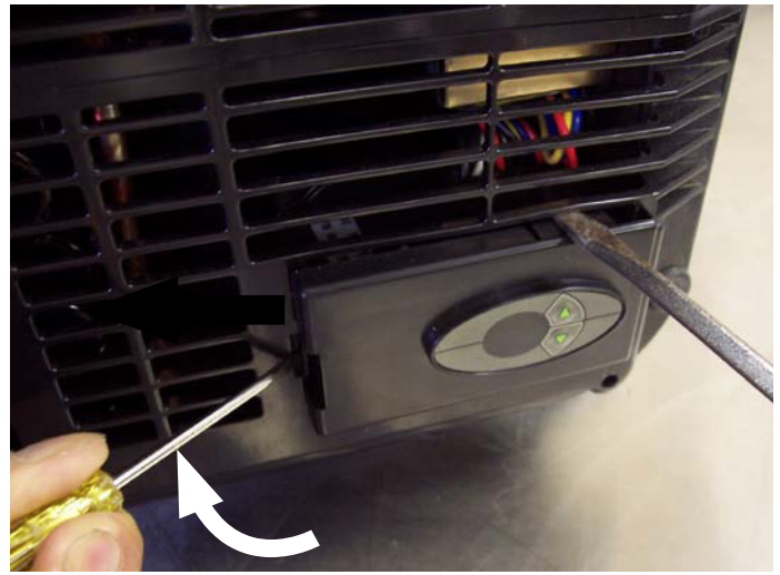
② Lever left snap fit tab out.
