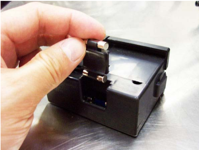
⑨ Remove fuse from NEW controller.
