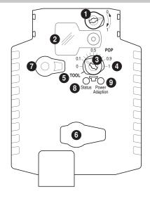
POP button 3 4 Scale for manual adjustment Position for adjustment with tool 5 6 Tool socket **Disengagement button** 7 LED displays Meaning / function 9 green 8 yellow Off Illuminated Operation OK / without fault Off POP function active Blinking Illuminated Off Fault Off Off Not in operation Adaptation procedure running Illuminated Illuminated Blinking Illuminated Communication with programming tool
