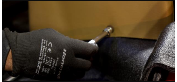
2 - M10 bolts on outer passenger side wall of storage bin
