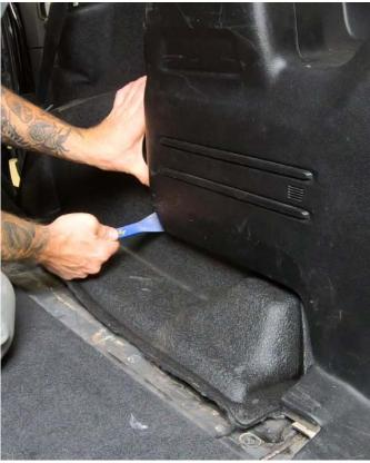
To ensure proper fit make sure the wheelhouse is tucked under the plastic and back far enough towards the rear of the vehicle. Example of subwoofer models. Installation is generally the same but the passenger wheel-house is shorter to accommodate subwoofer and trim.
