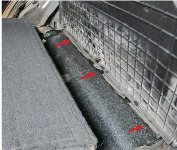
Closeout panel should overlap onto the rear floor, be sure to secure using the grommets provided.
