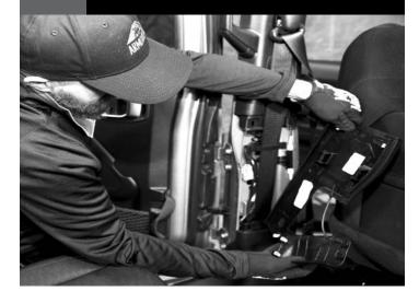
Remove battery close out trim underneath the rear seat; 3 pieces. Remove LH and RH corner trim pieces by unscrewing Torx screws (2 per side) and pulling up. Remove center trim piece by pulling forward.
