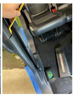
On these B pillar trim pieces there are 14 metal clips <u>between both sides</u>, make sure all of the clips are accounted for, if any are stuck back into the sheet metal, do not reuse them, instead use one of the replacements we provided. In our experience it is normal for 1-3 to come off the trim part and stay in the metal, we provided 7 to replace them since they are often unusable once they pull off the plastic.
