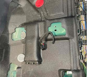
**20**. Run your hand around the perimeter of the floor and make sure it is down all the way and also not hung up on any components like wire harness connectors.
