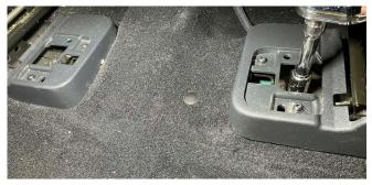
**2.2** Before unplugging, position the seat for better removal, moving it to the middle front to back position, seat height all the way down, and seat back leaned forward. Lay the seat back and unclip the harness from the seat by sliding the red tab (a.) back then depressing the tab (b.) to release. Seat is now ready for removal. Using painters tape, cover the door jam area to protect your paint. We also suggest a piece of cardboard over your
