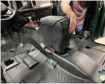
**18**. If equipped, place the vent through the opening in the floor.
