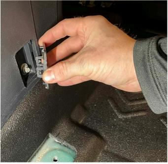
**26.** Place seat back into position and connect the harness. Then proceed to bolt down back into place. Be sure to replace plastic covers.
