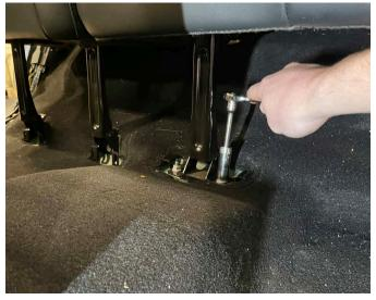
**11**. Fold the bottom of the seats up and secure with the seatbelt by pulling belt across seats, fastening in, then pulling the belt all the way out of the retractor then letting it pull back in locking in place. This should hold seats out of the way without the need for removing them.
