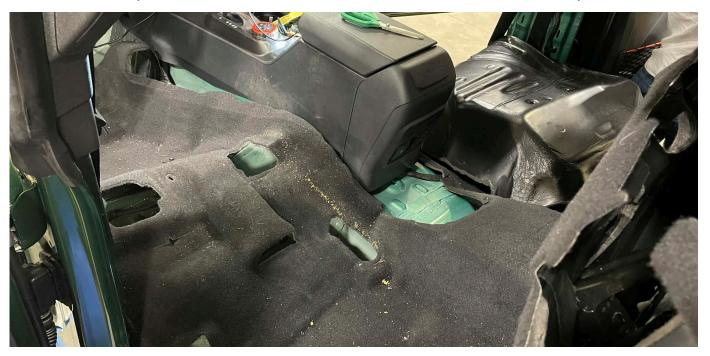
**15**. Locate the 4 factory plugs that match the 4 round plug openings in your Armorlite floor and remove them.
