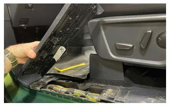
**4.** Remove the Driver side kick panel by first prying the cover off the dead pedal to access the nuts holding it in place.
