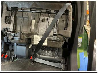
**12**. Check the perimeter of the floor and remove all other push pins or connectors
