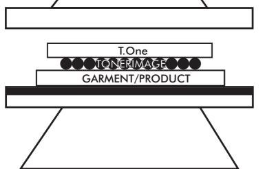
Note: Wait a few seconds before stripping off the base paper. Strip liner <u>right on the heat press</u> in one slow steady motion in a very shallow angle!
