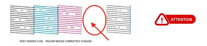
DO NOT DO ANY MORE CLEANINGS, OR FLUSHINGS while the printhead is in the printer. The printhead must be removed from the printer.
