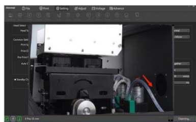
Step 17. And the waste ink will flow through the tube. The cleaning takes about one and a half minutes to finish.
