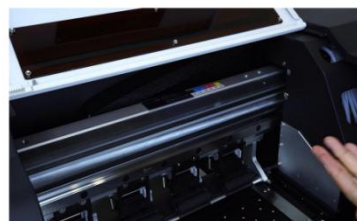
Step 4. The metal plates secure the drive belt during transportation but if you forgot to remove them before the machine is powered on, the drive belt could become deformed .
