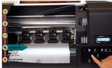
Step 1. Press the Left button on control panel.
