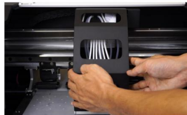
Step 4. Remove the black cover of the print-head assembly.
