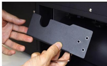
Step 12. The left side bracket is WITHOUT a bar holder.
