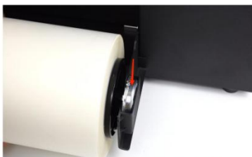
Step 25. Insert the bar holder into the right bracket slot completely.
