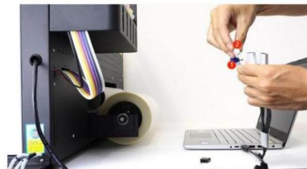
Step 4. Insert the two USB devices. ① The blue one is a RIP dongle, you'll need it every time you use the RIP software. ② The white one is a regular USB thumb drive stored with guidance videos and printer software.
