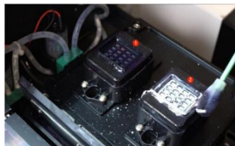
Step 15. Then we go on cleaning the two cappings. It's obvious that capping ① of color ink is more easily cleaned; capping ② is for white ink, on which residues will be more and be harder to be wiped off.
