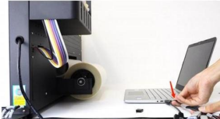
Step 5. Connect both USB devices to your computer. (As the picture shows, it's highly recommended to get a USB splitter to simultaneously function different drivers.)
