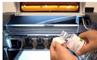
Step 5. Dip some ALCOHOL on lint-free cloth to start the cleaning.
