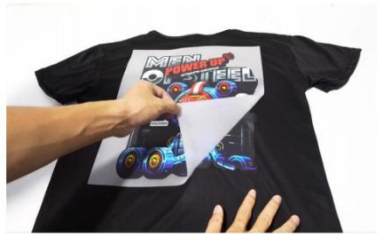
Step 21. And now you can peel off the film! Make sure to do the peeling gently and slowly
