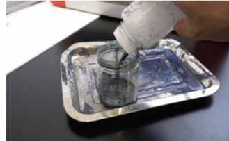
Step 2. Pour out the waste ink, ink waste bottle should be emptied regularly.
