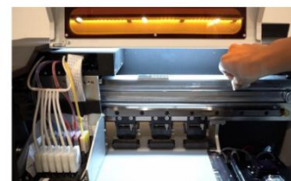
Step 8. Now go on cleaning the right side encoder strip.
