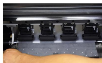
Step 37. Pull down the lever now to put the film advance array rollers down.
