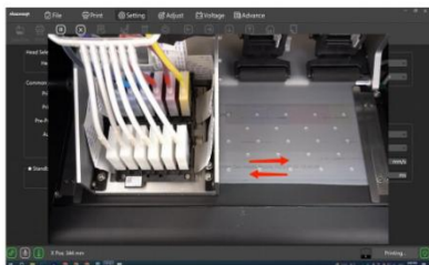
Step 19. During the checking process, the print head assembly will move back and forth and print a testing chart.
