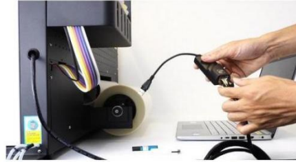
Step 2. Plug the printer cable into the USB adapter for fast data transfer. If your WAN port can reach the speed of 1 Gigabit per second, you don't need this USB adapter.
