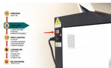
Step 50. Power on the printer. [the button situation in this picture means "off"]
