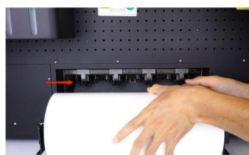
Step 35. Pass the film sheet through the array rollers.
