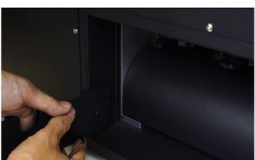
Step 13. Align the left bracket to the screw holes.
