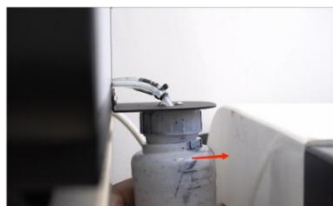
Step 3. Rotate counterclockwise to set the ink waste bottle back.
