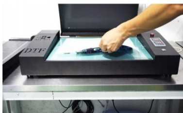
Step 11. Set the temperature at 120 degrees Celsius and the countdown timer to 180 seconds. Then gently put the film on the oven pad. [color side down]
