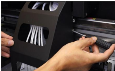
Step 3. Undo the screws at both sides.
