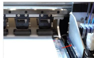
Step 10. And make sure the print head remains in the closed position on the capping station.
