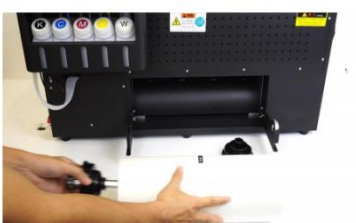
Step 20. Insert the roller bar through the film roll.
