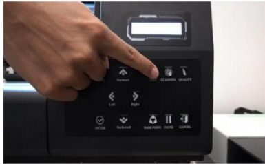
Step 1. Press test button on the control panel to initiate nozzle checking function.
