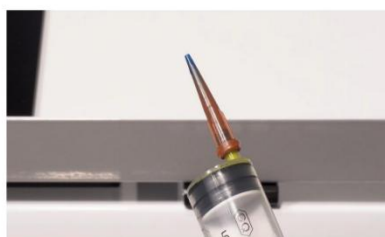
Step 9. Remember to change the needle hub for each ink to avoid color mixing.
