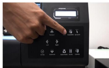
Step 8. When the cleaning is finished, press test button again.
