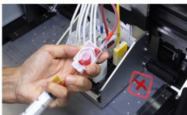
Step 7. Don't turn the ink cartridge downward when extracting ink, this will cause many bubbles in the ink.
