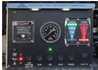
FoamPro® Foam Proportioning System installed on a Cascade Fire slip-on unit
