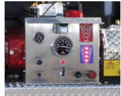
Intellitank Water and Foam meters, installed on an End Mount unit
