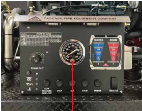
PRESSURE GAUGE ON A SLIP-ON UNIT SHOWS DISCHARGE PRESSURE AT THE PUMP
