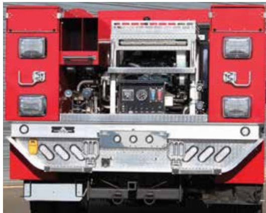
FoamPro® Foam Proportioning System installed on a Cascade Fire slip-on unit
