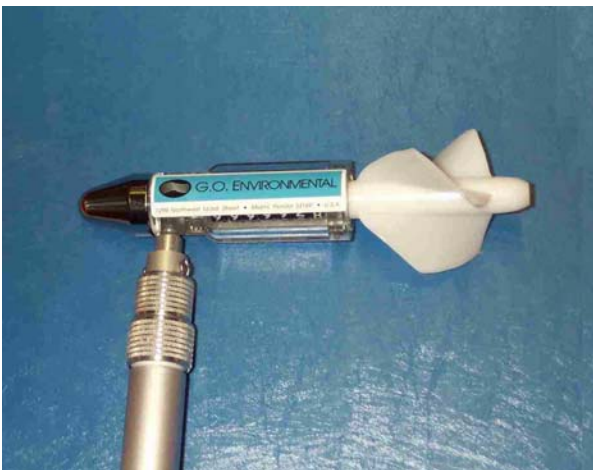
Model 2030R flowmeter with high speed impeller fastened to 2030W wading rod
