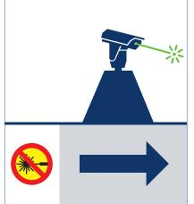
6. Select an installation location where the laser beam does not need to cross public roads, pathways, sidewalks or parking spaces in order to cover the intended bird zone.
