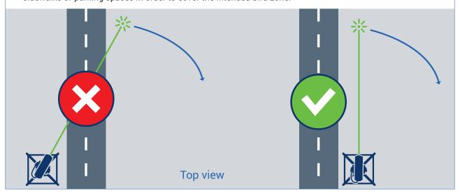
7. Where possible, position the Agrilaser Autonomic at increased height with respect to the surface of the bird zone.
