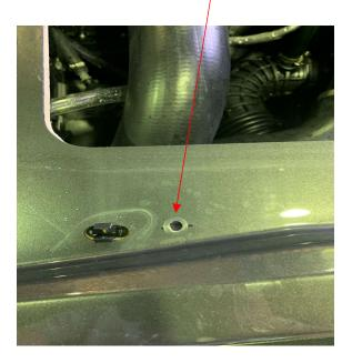
Install the 4-inch adapter using the left threaded hole as per Diagram to the mounting bracket
