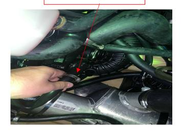
3 Loosen hose clamp and pull hoes off supercharger
