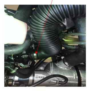
Fasten the other side of the flexible hose to the air filter adaptor and mount the adapter to the hull
