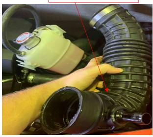
Fit supercharger adapter
