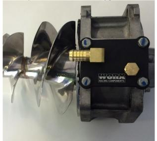
Fit ½ inch fitting to cooling plate with sealant. Drill 16mm hole thru transom to fit ½ inch thru hull fitting. Fit with sealant. (Thru hull fitting is best fitted towards the top of the tunnel). Either left or right side on FZ models and FX non RiDE models and centre on FX SVHO RiDE models. Make sure inside ski is clear before drilling.)
