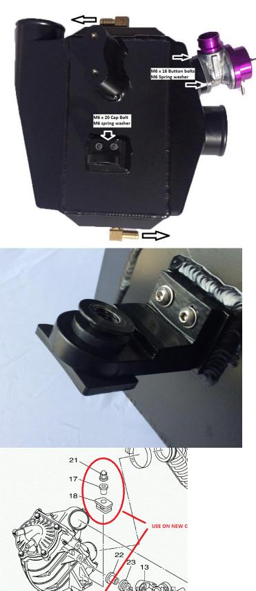
6- Remove jet unit and fit new cooling plate to side of the jet unit.
