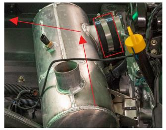
**22.** In the pump tunnel, remove the steering connection, using a 10mm spanner & socket.
