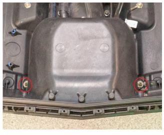
**28.** Using a flat bladed screwdriver or prying tool, beging to carefully pry the ride plate from the hull. Depending on the amount of OEM sealant, some force may be required.
