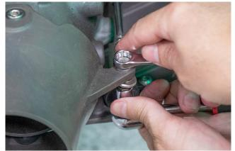
**23.** Disconnect the hose clamp and disconnect the bilge pump hose.
