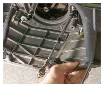
**29.** Once the sealant releases, pull the ride plate towards the back of the hull and remove. Clean the hull of any sealant residue and ensure the hull is as clean as possible from dust oir debris before continuing.
