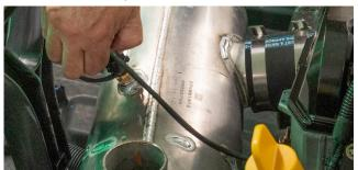
**20.** Remove the sensor from the waterbox using a 19mm spanner.
