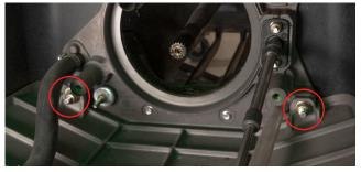
**27.** Undo the 2 x nuts picture below and retain bolts and washers.
