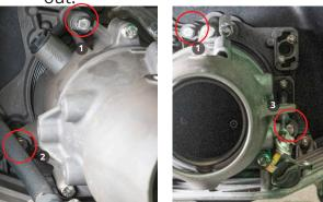
**25.** Undo the 4 x Torx bolts connecting the hoses to the ride plate.
