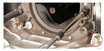
**32.** Reinstall the rear two bolts and nuts securing the back of the ride plate to the hull.
