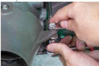
**23.** Disconnect the hose clamp and disconnect the bilge pump hose.
