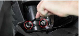
6. Undo the 10mm nyloc nut and bolt, connecting the steering arm to the clamp.
