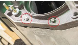
**32.** Firmly tighten the other three bolts pictured below and replace the red cap on the left bolt.
