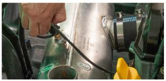
**20.** Remove the sensor from the waterbox using a 19mm spanner.
