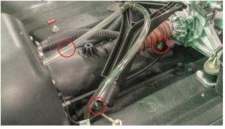
33. Clean any sikaflex that has seaped out. Work in reverse from step 24 to reinstall all connections and top deck. Ensure all connections are tight and secure before reconnecting battery and testing part.
