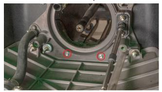
**26.** Remove the 3 x bolts pictured below. Retain the red cap on the left bolt.
