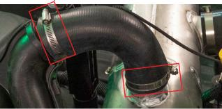
**19.** Unclip the exhaust temp sensor and cut the zip ties.
