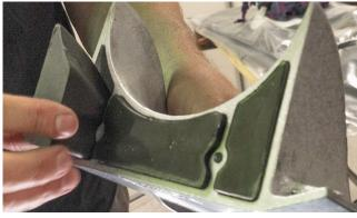
**29.** Apply marine sealant as pictured below. It is better to apply an excess in order to reduce air pockets and
