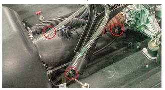
**27.** Using a flat blade screwdriver, pry the OEM intake grate from the hull.
