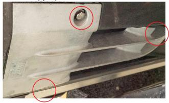
**31.** Use the provided bolts to secure the back of the intake grate, as pictured
