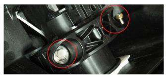
**9.** Pull the steering column up and away from the ski, whilst feeding the cables back through the column as you pull it away.
