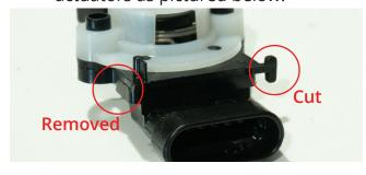
**24.** If the spring falls away from the unit, replace the locating tabs in the positions show in the images below.
