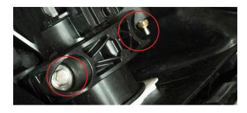
**13.** Re-clip in the dash plate cover and secure using the OEM torx bolts.
