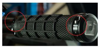
**20.** Undo the bolts securing the Electronic Throttle and IBR actuator units in place and both levers using a 5.5mm or 7/32" socket & 8mm socket.
