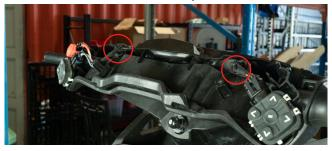
4. Remove the back handlebar cover plate by using a flat bladed screwdriver to gently pry the cover plate away from the lower assembly. Clip locations can be viewed below.
