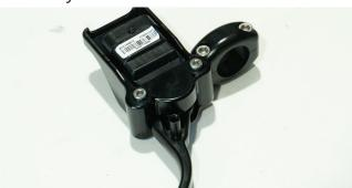
**28.** Clamp the lever housing to the handlebar using a 4mm hex key.
