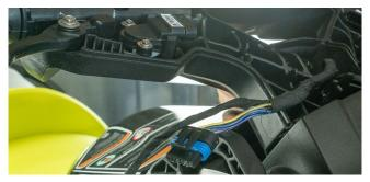
Undo the plastic lock nut securing the DESS post in place and unclip the DESS post cable. Retain the lock nut and pull the cable through the back of the steering column.
