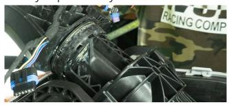
**10.** Remove the top bush from the steering column and fit to the supplied Worx steering column as pictured.
