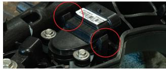
**22.** To assemble the throttle and IBR assemblies, remove the white spacers from the units.
