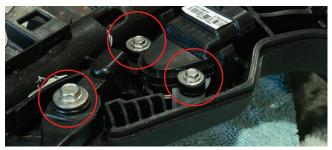
**21.** Unclip the two retaining clips holding the actuators in place and remove from the OEM handlebar assembly.
