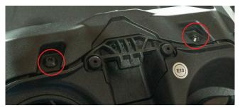
**8.** Undo the two bolts securing the steering clamp retainer piece using a 10mm socket.
