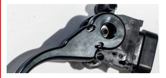
27. Place the actuator and trigger into the lever housing as pictured below and secure using housing top clamp and bolts provided, using a 3mm hex key.
