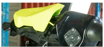
2. Using an 8mm Socket, remove the two bolts picture and removed the plates covering the switches.
