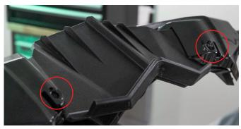
**9.** Remove the torx bolt located under the panel at the front of the steering and remove the panel.
