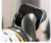
**28.** Attach your throttle lever. Test the angle whilst sitting on your ski, before securing and reconnecting the wiring.
