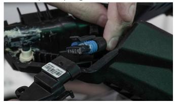
**14.** Unclip and remove the start/stop switch button.
