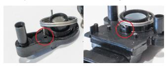
**19.** Place the washer on the small protrusion from the top side of the lever housing.
