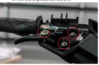
**12.** Carefully remove the throttle lever.
