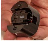
22. Remove the top bush from the steering column and fit to the supplied Worx steering column as pictured.
