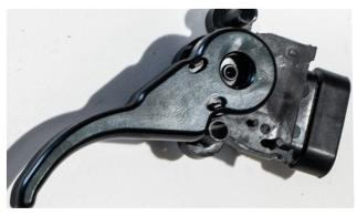
21. Place the actuator and trigger into the lever housing as pictured below and secure using housing top clamp and bolts provided, using a 3mm hex key.
