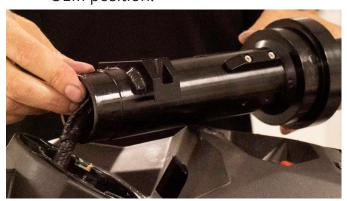
**24.** Secure the steering stem to the OEM steering clamp backing using the supplied M6 x 35mm bolts.
