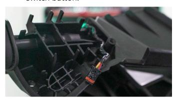
**15.** Feed wires through the center and pull the steering stem up and out of the ski.
