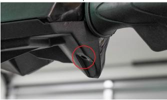
**10.** Unclip the top cover of the start/stop button housing and the throttle level switch cover.
