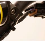
**29.** Use zip ties and cabling to secure wires neatly around the bars.
