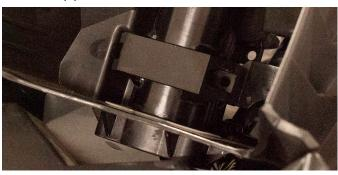
25. Place the bars between the clamps and begin to secure the bolts evenly. Ensure that all of the bolts are secured and the gap between the clamps are all even.
