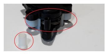
**17.** Cut the tabs on the outside of the actuators as pictured below.
