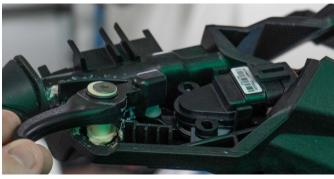
13. Unclip and remove the throttle actuator housing, being careful to hold the assembly together so you don't drop the spring.
