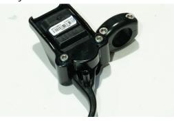
**22.** Place the button from the start/stop switch into the Worx holder and then carefully placed switch into the holder as pictured.
