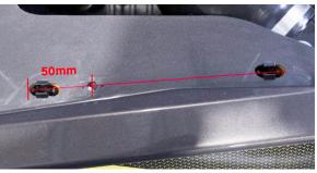
**9.** Secure your bracket and pod to the hull using the provided M6 bolt, nut and washer. Finally secure the adaptor to the silicon hose using supplied Hose clamp.
