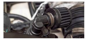
**6.** Fit the supplied silicon hose to the supercharger using the OEM hose clamp.
