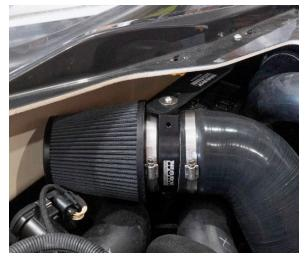
**10.** Ensure all connections are tight and secure before reinstalling all panels and seat.
