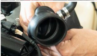
**17.** Undo clip and throttle body wiring connection pictured below.
