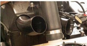
**21.** Fit the pod filter to the other end and secure with supplied hose clamp.
