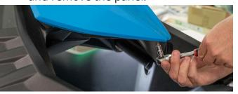
**5**. Undo the steering clamp by removing the 2 x 10mm bolts.
