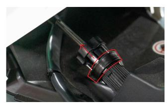
**9.** Undo the connection by spinning clockwise until it's removed.
