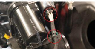
**18.** Secure the reducer hose to the throttle body connector using supplied hose clamps.
