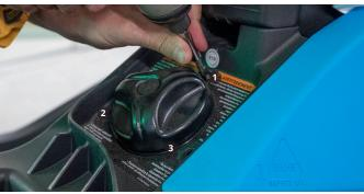
Remove the torx bolt located under the panel at the front of the steering and remove the panel.
