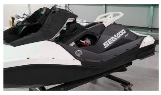
**14.** Remove the hull lifting up and toward the front of the ski so that the steering arm slides through the grommet.
