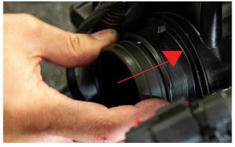
**24.** Reinstall throttle body connector and use supplied hose clamp to resecure.
