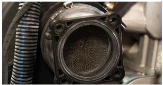
**21.** Using needle nose pliers or a flat blade screw driver, gently pry the rubber ring and ribbon from the inlet manifold, being careful not to damage it as you will need to reuse the OEM rubber.
