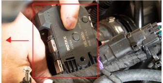
**20.** Undo hose clamp and remove throttle body connector..
