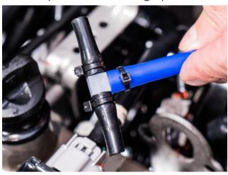
**9.** Reinstall the map line between your manifold and map sensor. Secure using zip ties.
