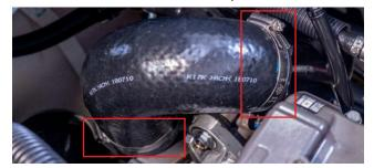
3. Secure the replacement Blow Off Valve (BOV) hose using the OEM hose clamps. Ensure the end of the hose used to secure the BOV unit is facing towards the centre of the ski, as pictured below.
