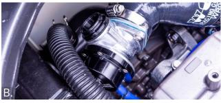
5. Secure the 1m of BOV Hose Line to the Vacuum Nipple using a supplied zip tie.
