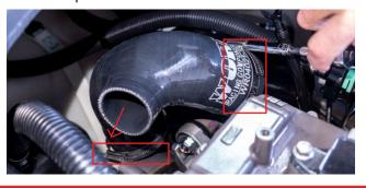
4. Fit the BOV unit the to intake hose using the 1½" hose clamp provided. Please Note: We recommend fitting the BOV Unit at a 30° Angle as pictured (A) or 150° Angle (B).
