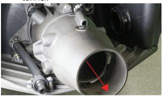
Remove the wear ring from the tunnel.
