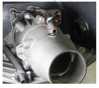
4. Remove the three bolts pictured below before pulling the pump unit
