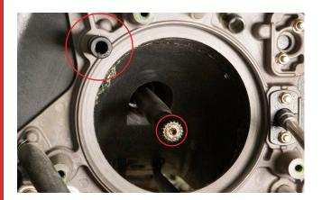
**11.** Reconnect the water line and reinstall the three bolts from step 4.
