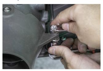
Disconnect the hose clamp and 3. disconnect the bilge pump hose.
