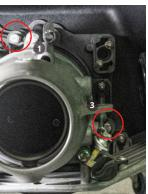
Pull the pump out through the tunnel.
