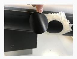
4. OPEN THE GLUE, AND APPLY THE GLUE WITH A BRUSH ON THE PATCH AND AROUND THE HOLE.
